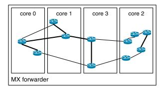
Figure 2: An example showing possible allocation of routers to CPU cores in MX.
