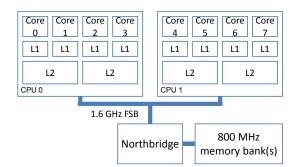
Figure 3: CPU and memory architecture of the Intel SR1560 server.
