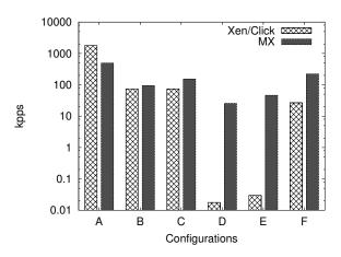
Figure 4: Comparison of scalability of Xen/Click and MX under different configurations (y-axis is in log-scale).
