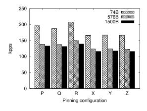
Figure 6: Throughput of the same MX configuration with 4 routers, using different router-to-core pinnings.
